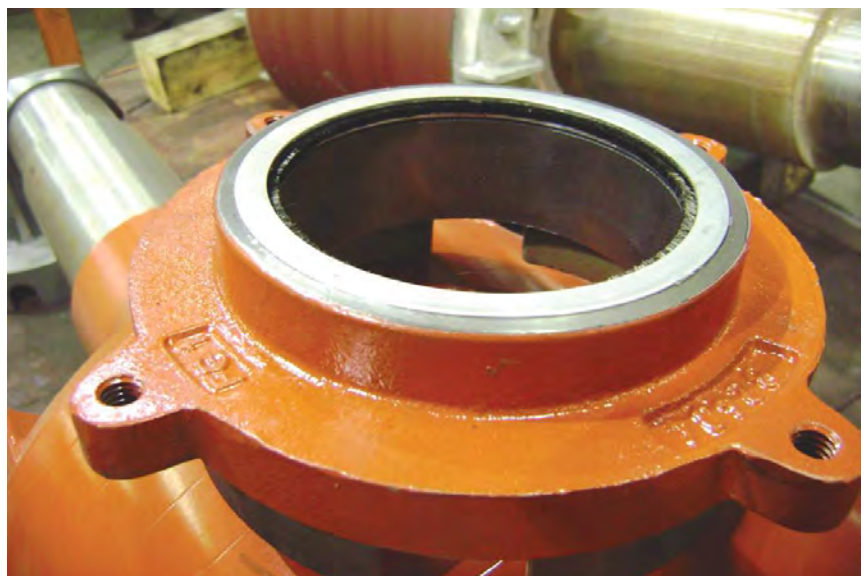
Figure 5: For internal installation, the grounding ring is often mounted in a bearing retainer.
