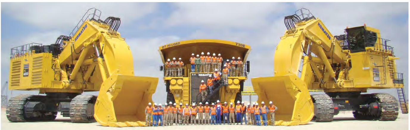
The team of mechanics responsible for looking after two Komatsu PC 4000s and a fleet of 730E haulers at Vale's Bayóvar phosphate mine in Peru. Weighing in at 390 mt (430 ton), these PC 4000s carry a 29 m 3 bucket because of the low density of the rock.
