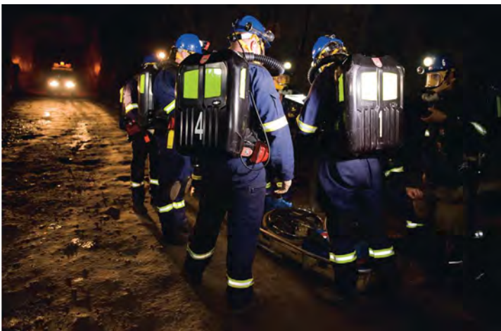
Dräger’s closed-circuit breathing apparatus offers a four-hour working duration.
