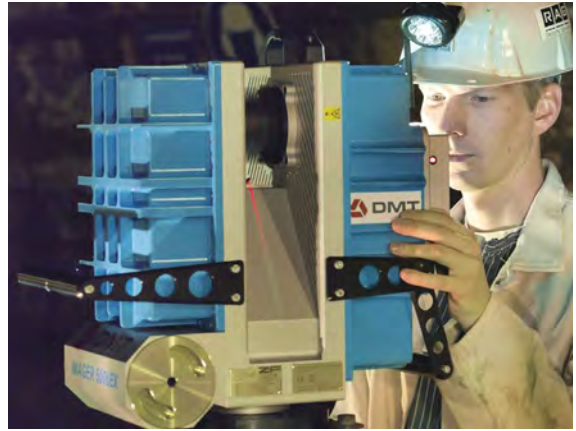
The world's first explosion-proof 3-D laser scanner, developed by DMT.
