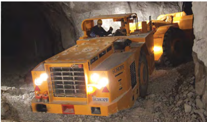
Schopf's SFL 140 LHD, designed to work with 40- to 50-mt capacity trucks, has a 250 kW Tier 4A (Stage III B) engine.
