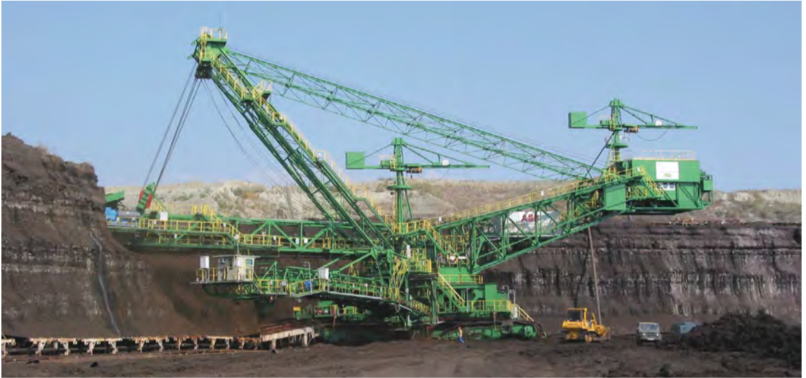
ABB supplied retrofit drive technology for this SchRs 1200 bucket-wheel excavator in Bulgaria.
