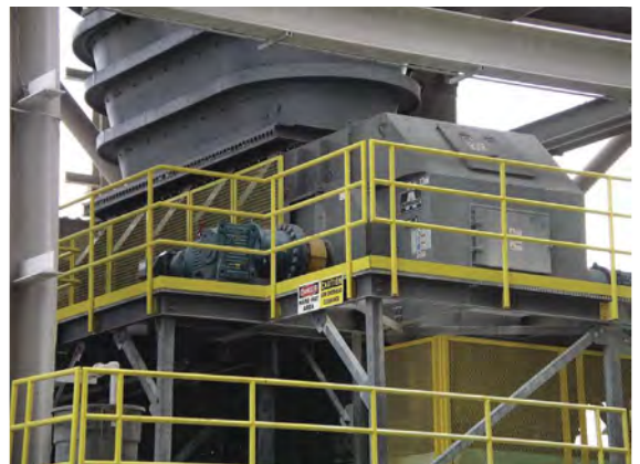
A BPB-type apron feeder from Aumund, designed to handle moist or sticky materials.
