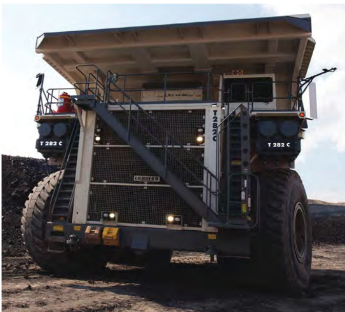
Liebherr's flagship truck, the 363-mt capacity T 282 C.
