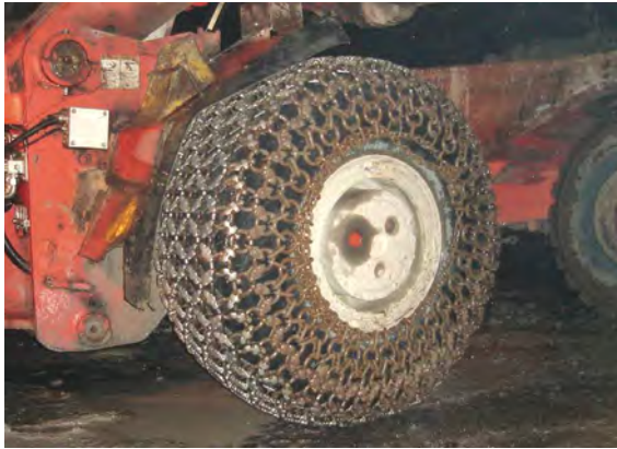
Erlau tire-protection chains provide comprehensive protection in the toughest mining environments.
