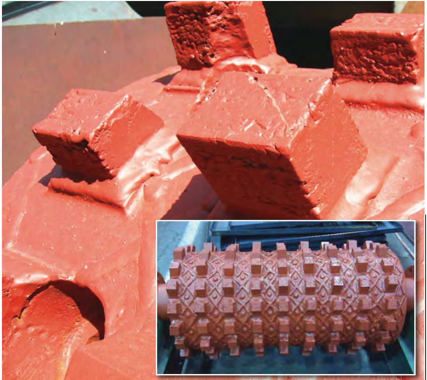
McLanahan's new weld-on carbide teeth allow miners to make repairs rather than replacing the roll segment.
