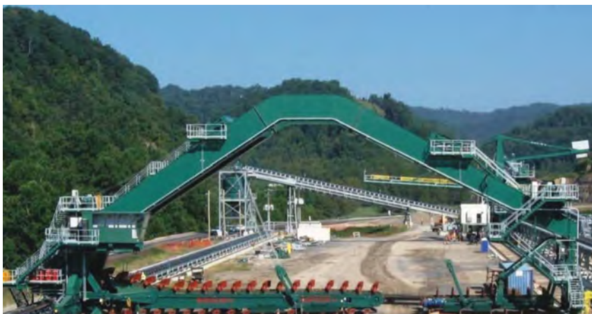
Rake reclaimers will pull coal from a high- and low-grade area.
