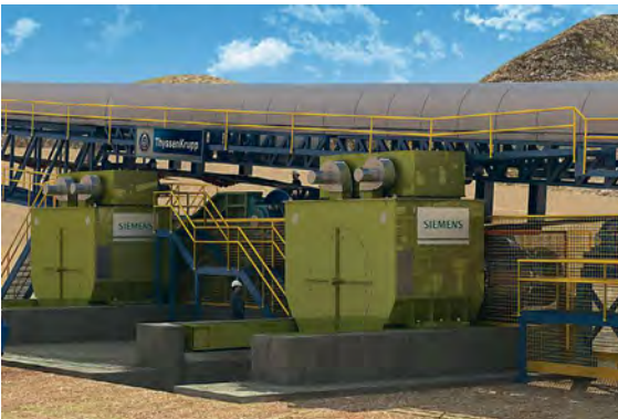
Gearless drives offer significant advantages in high-capacity conveyor applications, according to Siemens.
