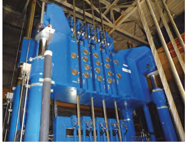
A Siemag Tecberg clamping and lifting device, used for shaft rope changing and maintenance.
