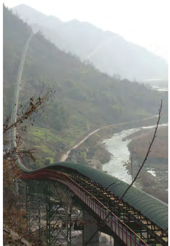
Beumer specializes in designing and building curved belt conveyors.
